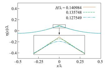
**Fig. 2.** (Color online) Stokes wave for 1.082500 (blue line), 1.091500 (green line), and  $c/c_0=1.0922795$  (dark orange line). Corresponding values of  $H/\lambda$  are given in the legend. Inset shows zoom-in into small values of  $x/\lambda$  near a wave crest.
