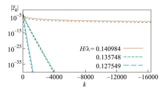
**Fig. 3.** (Color online) Spectra of Stokes waves for the values of  $H/\lambda$  as in Fig. 2 (thick lines) and fit to (14) with  $\beta = 1/2$  (thin dashed lines). Solid line shows only a small fraction of the actually numerically resolved spectrum.
