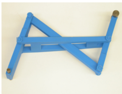
Figure 1: Dynamically balanced planar four-bar mechanism (Gabriel's Mechanism, [5])
