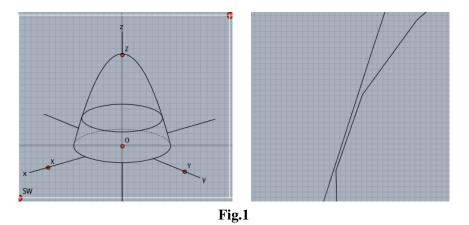
To refine the calculation of item 2, we have adopted an interpolatory scheme using Bézier curves near the contact point. Then we use a formula developed by Oshima[1] to decide the control points.
