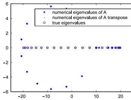
Fig. 5. Numerical spectra of  $A$  and  $A^T$ ,  $n = 20$ ,  $a = 100$ , obtained by routine DLAHQQR.
