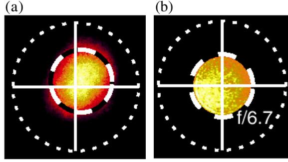
**Figure 3.** Experimental images of the cross section of time averaged laser beam intensity after propagation through plasma. (a) Onset of beam spray regime at  $5 \times 10^{14} \text{ W cm}^{-2}$ . (b) Negligible beam spray regime achieved by lowering intensity. The dashed circles correspond to  $F = 6.7$  beam width for propagation in vacuum. Reproduced from [8] with permission.
