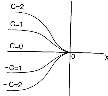
2. Diagonalization yields a system of the form  $\dot{x} = \alpha(x + y)^2 - y(x + y)$ ,  $\dot{y} = -y - \alpha(x + y)^2 + y(x + y)$ ; then from (5),  $h(x) = -\alpha x^2 + \alpha x^3 + \dots$  and on  $W^c(\mathbf{0})$ ,  $\dot{x} = \alpha x^2 + O(x^3)$ ; so for  $\alpha \neq 0$ ,  $\mathbf{0}$  is a saddle-node. For  $\alpha = 0$ ,  $h(x) \equiv 0$  and the x-axis is a line of critical points.
