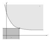
roughly,  $x_0$  Pareto optimal means  $F(x_0)$  is on tradeoff surface  $(F(x_0) \in \partial A)$
